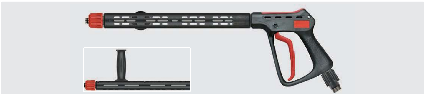
Professional ultra high pressure gun with extension ST-9 380 mm, grip and quick screw coupling ST-740. Max. 600 bar / 80 l/min / 150 °C
