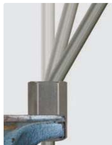
Stainless steel. Lance bender for 1/4" M lances without nozzle protector
