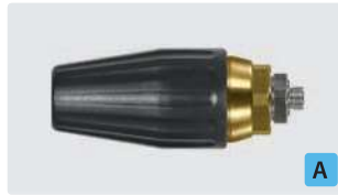
1/8" M. Spray angle 20°. 100 - 250 bar. Max. 100 °C
