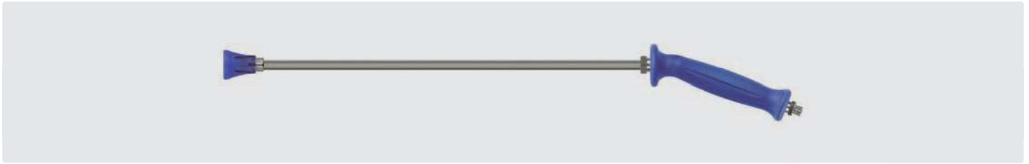
Stainless steel. Lance with easywash365+ handle and nozzle protector ST-10 without nozzle. Max. 350 bar / 45 l/min / 150 °C
