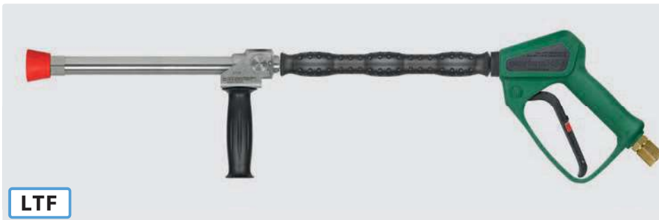
1/2" F. Stainless steel. Longcast lance 350 mm with insulation ST-29 Cool & Compact 330 mm, gun easyfarm365+, grip aside and nozzle protector made out of plastic without nozzle. Max. 250 bar / 60 l/min / 100 °C
