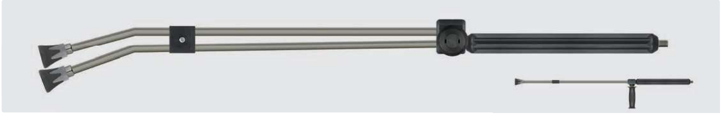
1/4" M. Lance with moulded handle, valve ST-54 aside and nozzle protector ST-10 with low pressure nozzle & thread 1/4" F. Max. 310 bar / 150 °C
