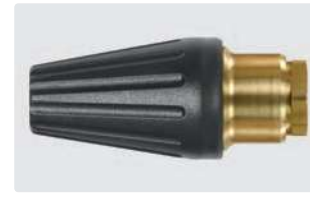
1/2" F. Spray angle 20°. 120 - 250 bar. Max. 100 °C
