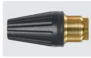
1/2" F. Spray angle 20°. 120 - 250 bar. Max. 100 °C
