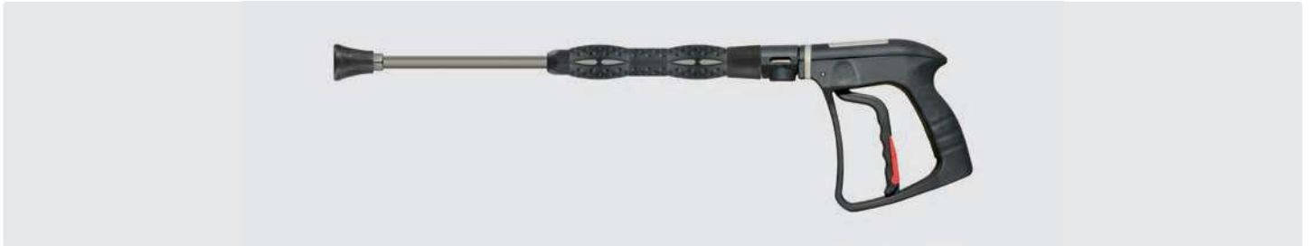
Professional steam gun with lance stainless steel 400 mm, vented handle ST-9.1 220 mm and nozzle protector ST-12 without nozzle. Max. 20 bar / 200 °C
