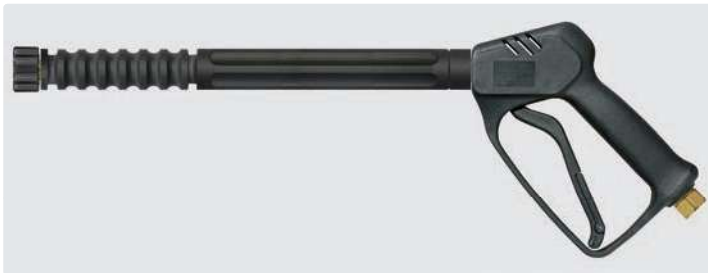
Professional gun with extension 340 mm and M22 F. Max. 210 bar / 25 l/min / 150 °C
