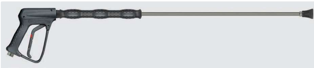
Professional gun R+M EcoLine No. ONE with lance 900 mm zinc-plated steel, insulation ST-28 Cool & Compact 300 mm and nozzle protector ST-10 without nozzle. Max. 250 bar / 45 l/min / 150 °C
