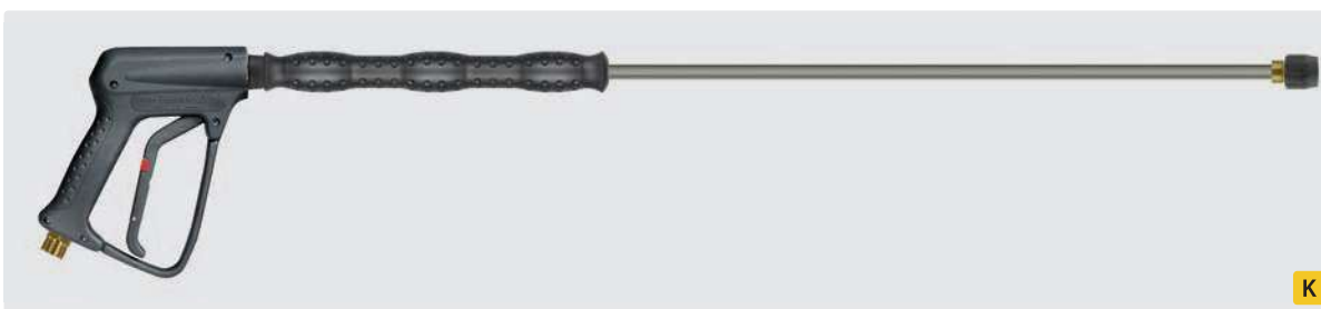
Professional gun R+M EcoLine No. ONE with lance 900 mm zinc-plated steel, insulation ST-28 Cool & Compact 300 mm and nozzle protector without tip. Max. 250 bar / 45 l/min / 150 °C
