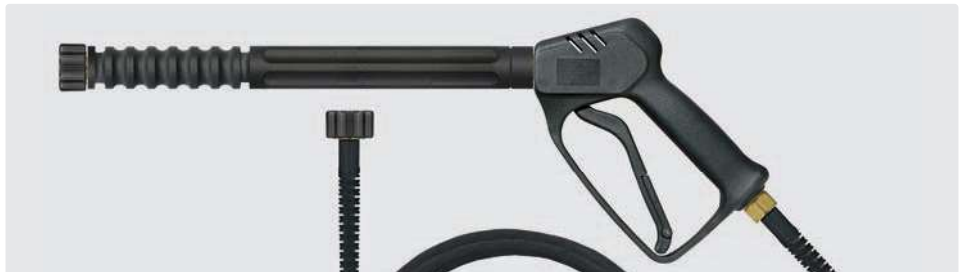
Professional gun with extension 340 mm, max. 210 bar / 25 l/min / 150 °C. Inlet / outlet M22 F. Hose: 6 - 160 (polyester interior), max. 160 bar / 20 °C
