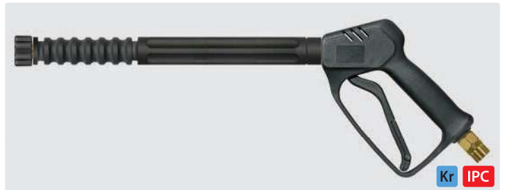
Professional gun with extension 340 mm and M22 F. Max. 210 bar / 25 l/min / 150 °C
